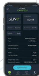
The WAYVE app, for programming opening times, automatic leak detection, system control, collecting historical and statistical data, and geolocating the box
