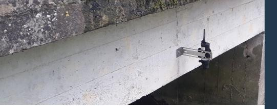
Installation of measuring instruments to monitor water tables
